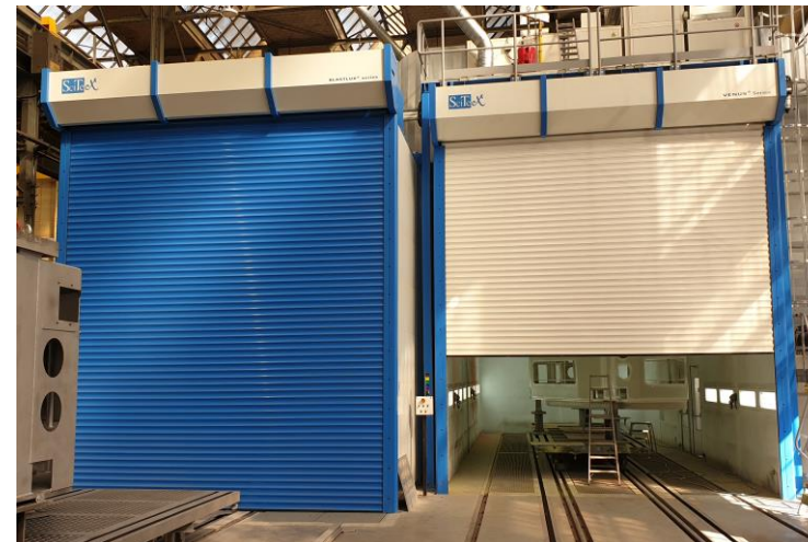
SciTeeX shot blasting & painting facility
